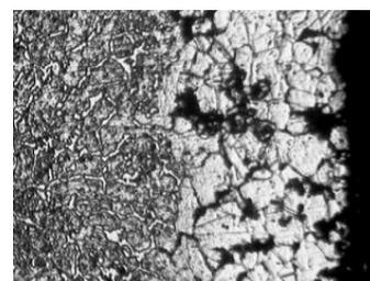
outer diameter and progressing towards ID. This magnification was done at the TCR Engineering laboratory using a Leco Image Analyser at 300X.
